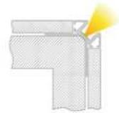
**Abdeckung** | PMMA - Polymethylmethacrylat
